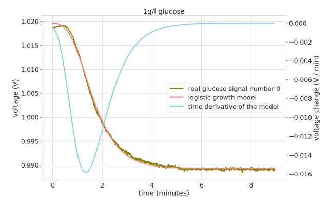
The green curve is the actual measurements of the glucose sensor. The orange curve is a generalized logistics growth model that is fitted to the sensor data.
