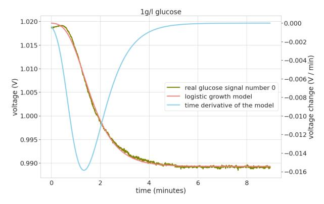
The green curve is the actual measurements of the glucose sensor. The orange curve is a generalized logistics growth model that is fitted to the sensor data. This model gets all the sensor measurements to fit a model. The idea would be to get the final voltage much earlier.
